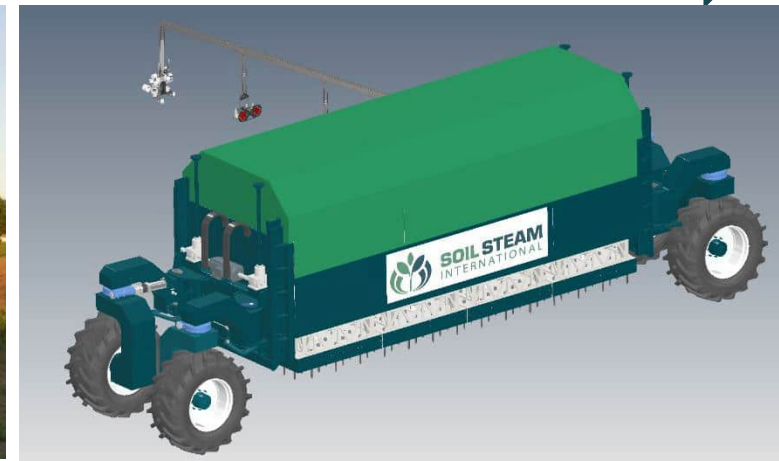
Prototype 4. Steaming cost and efficiency expected to be competitive to existing chemical solutions.
